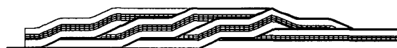
Fig. 9. Duplex structures with a planar roof thrust, modeled with our algorithm, where the thrust ramps are composed of various segments or have steps at several stratigraphic levels. The model parameters are u/s = l/s = 1/2 . The results indicate that the equations derived in this paper for the formation of duplexes with a planar roof thrust are independent of the ramp geometry. Further explanations in the text.
