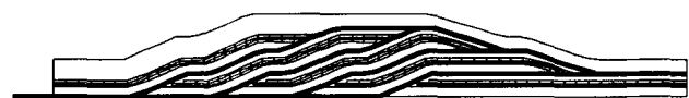
Fig. 1. Examples of duplexes with a planar roof thrust modeled with a kinematic algorithm that assumes displacement of constant length, parallel to the underlying active fault segment, for all the displaced particles throughout the medium (Fig. 2). For the definition of the duplex parameters ( u : displacement along the ramps, l : ramp length, and s : separation between the ramps in the undeformed state) see Fig. 3. The ramp series has a constant dip and spacing in the undeformed state, and the deformation sequence is in the direction of tectonic transport, with equal displacement along each ramp.
